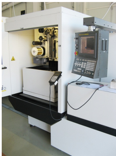
Wire-cut Machining Center FANUC ROBOCUT α-0iC Stroke X320 x Y220 x Z255mm angle up to 30° UV-axis á 120mm
