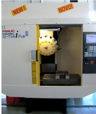
Small Machining Center FANUC ROBODRILL α-T14iFLe Stroke X700 x Y400 x Z330mm
